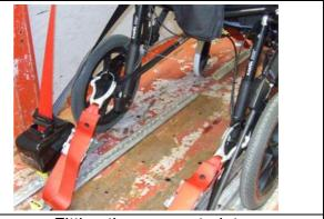
Fitting the front restraint
